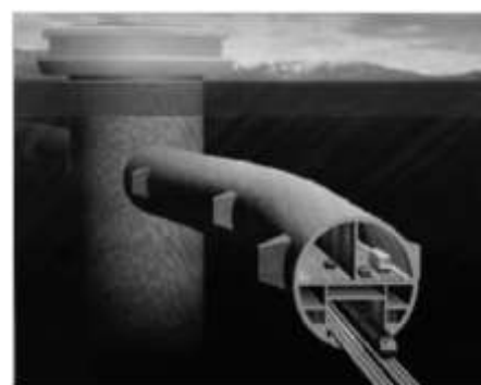
Fig. 2 Conceptive figure of submerged floating tunnel for the Funka Bay (Kanie S., (2010))
