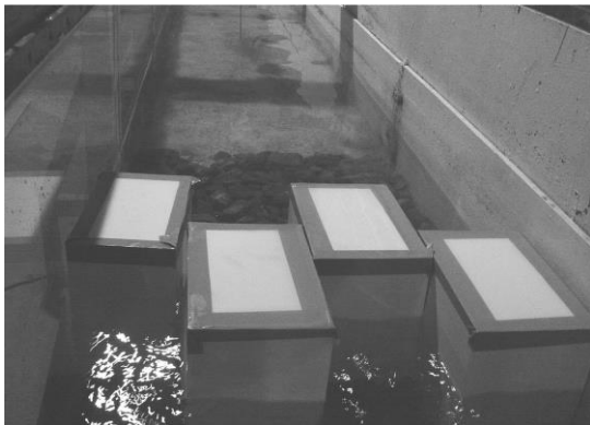
Fig. 6 Behavior of caissons in Case 1 at the incidence of approximately 250 waves of H_{1/3} = 6.8 cm and T_{1/3} = 1.7 s, taken from the offshore side
