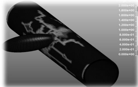
Fig. 8 Crack strain distribution after 1 sec impact
