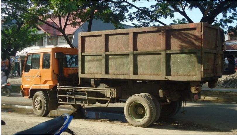
**Gambar 4.2** Arm roll truck berkapasitas 10 m<sup>3</sup>
