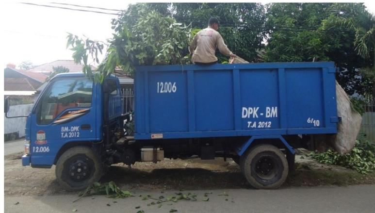
**Gambar 4.1** *Dump truck* berkapasitas 6 m<sup>3</sup>
