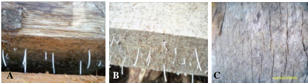
Fig.10. Degradation of wood and Frass Produced by Lyctidae: (A) frass of Anisoptera spp ; (B) Frass of Vatica spp ; (C) The exit hole on P.falcataria .
