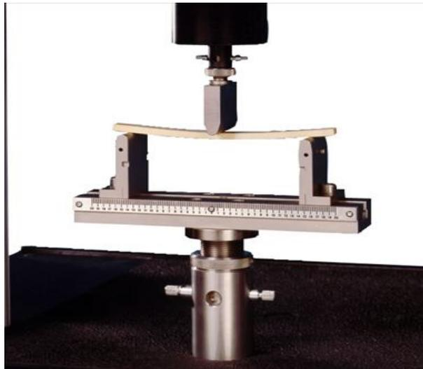
**Gambar 6. *Three Point Bending***
