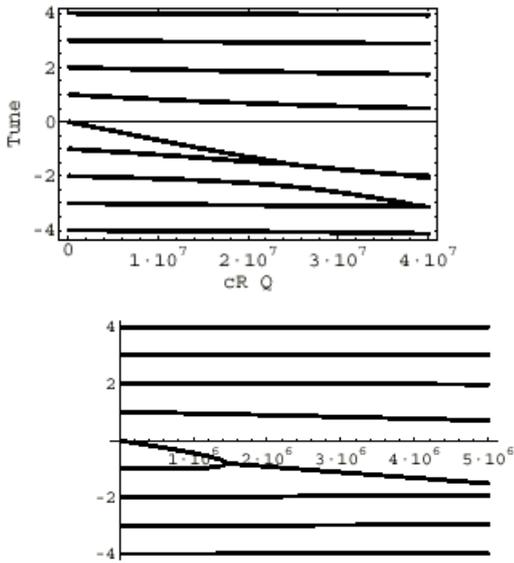
Figure 3: Horizontal mode coupling due to the e-cloud wake field in dipole magnetic field for KEK LER (above) and SPS (bottom)
