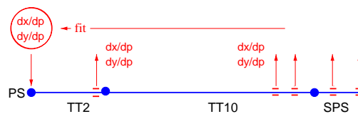
Figure 1: Schematic representation of the dispersion measurement
