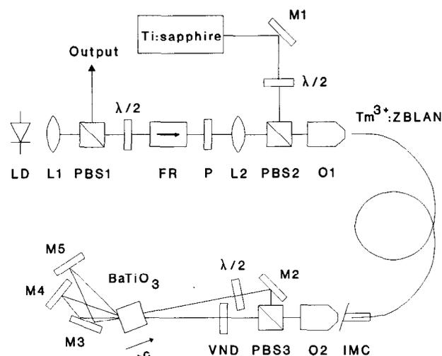
Fig. 1. Experimental arrangement. LD, laser diode; L1, lens (focal length 6.5 mm); PBS's, polarizing beam splitters; FR, Faraday rotator; P, polarizer; L2, lens (focal length 100 mm); O1, 10× microscope objective; O2, 20× microscope objective; IMC, index-matching cell; VND, variable neutral-density filter; M's, mirrors.
