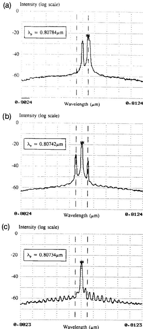
Fig. 3. (a) Optical spectrum at output under feedback conditions with diode blocked and with a notch filter in the ring cavity, and (b) the same arrangement 10 s later. Note the peak separation of  $\sim 0.5$  nm. The dashed vertical lines mark peak positions. (c) Spectrum showing diode mode separation of  $\sim 35$  nm. Note that the peaks in (a) and (b) do not appear to correspond to the modes of the laser diode.  $\lambda_p$  indicates the peak wavelength.
