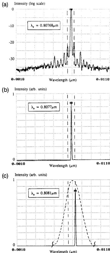
Fig. 2. Optical spectrum at output under feedback conditions with (a) diode present (log scale), (b) diode present (linear scale), and (c) diode blocked. The dashed curve (short dashes) is a schematic representation of the bandwidth calculation, and the dashed vertical lines mark the peaks of the modes adjacent to the fundamental diode mode.  $\lambda_p$  indicates the peak wavelength.
