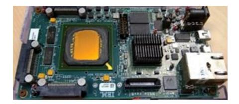
Fig. 6. Picture of the TrueNorth board after the chip (middle-left) was delidded.
