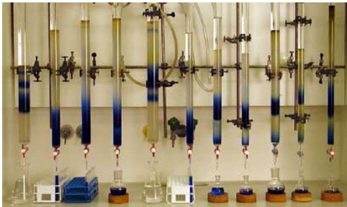
Figure 3.2: Application of the CSP methodology allows for visual tracking of the separation process during preparative column chromatography and, additionally, the isolation of target compounds is facilitated. 61
