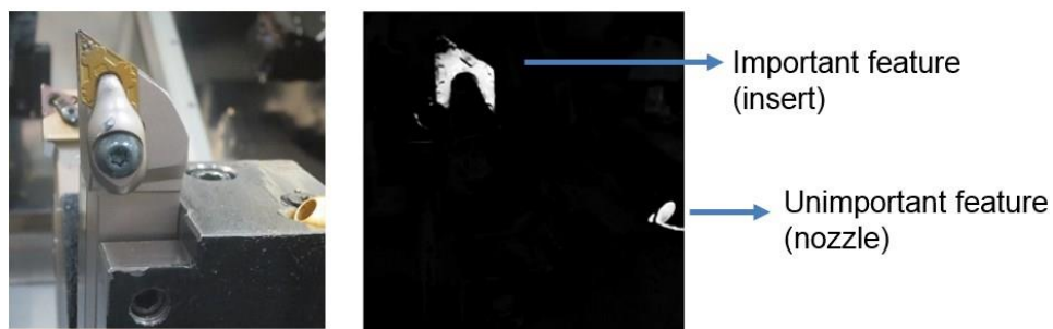
Figure 4.3 Detected features of a tool by the convolutional layer
