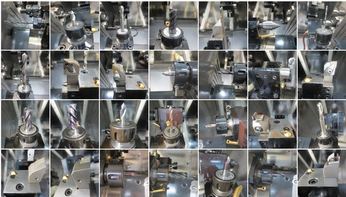
Figure 4.1 Installed tools in Nakamura-Tome turning-milling machine
