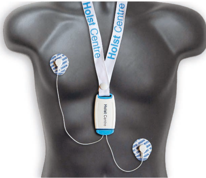
Figure 1-1: ECG sensor [ https://www.koenenco.nl/wp-content/uploads/2015/08/JM-01-webiste-04.jpg ]
