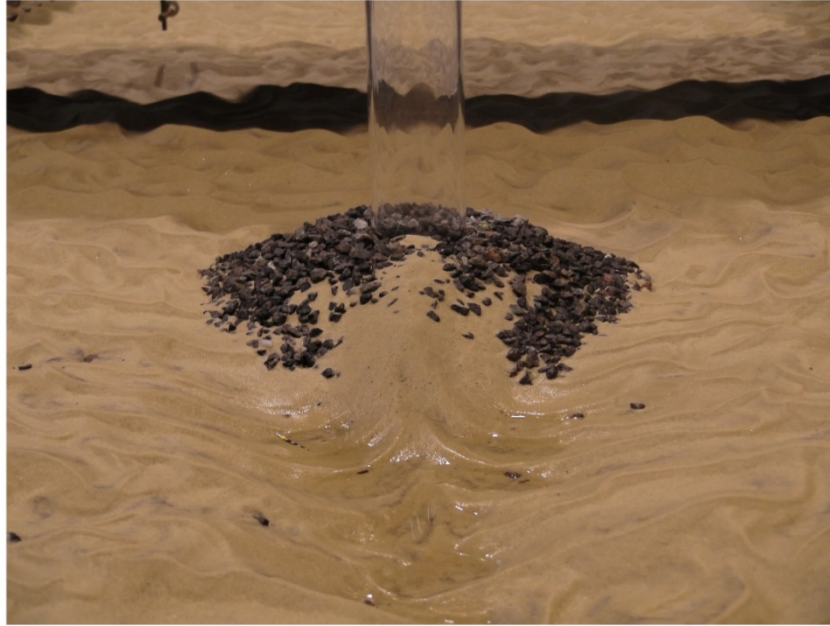
Figure 3.18. Image taken downstream of the bottom-mounted cylinder with scour protection, facing upstream (Test 23, Table 3.1).
