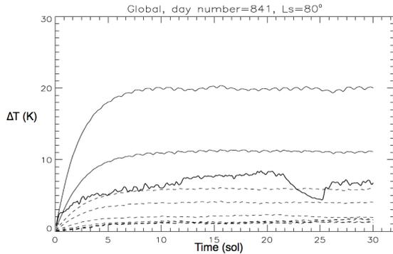
Figure 4: Time series of the growth of model error starting from an initial assimilated state at  $L_S = 80^\circ$  in MY25. The thick solid line represents the rms temperature difference at 30 Pa between uncorrected model forecast and the corresponding assimilated analysis, while other curves represent 'corrected' forecasts with differing values of  $\tau$  ranging from  $< 1$  sol (solid lines) to  $> 1$  sol (dashed lines).
