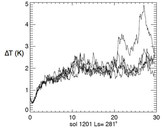
Figure 1: Growth of ensemble spread in terms of rms temperature differences between ensemble members on the 30 Pa pressure surface, averaged over the globe. Example shown for  $L_s = 281^\circ$  in MY25.
