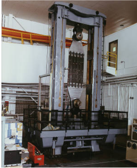
Figure 22a. Stitched/RFI wing panel in Langley 1,200-kip machine for discrete damage tolerance test.
