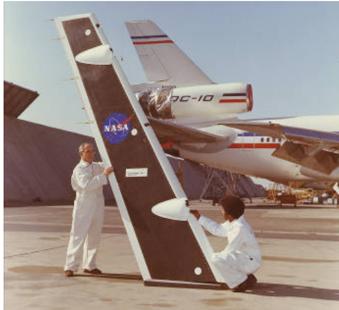
Figure 1. Carbon-epoxy upper aft rudder for DC-10 transport aircraft.
