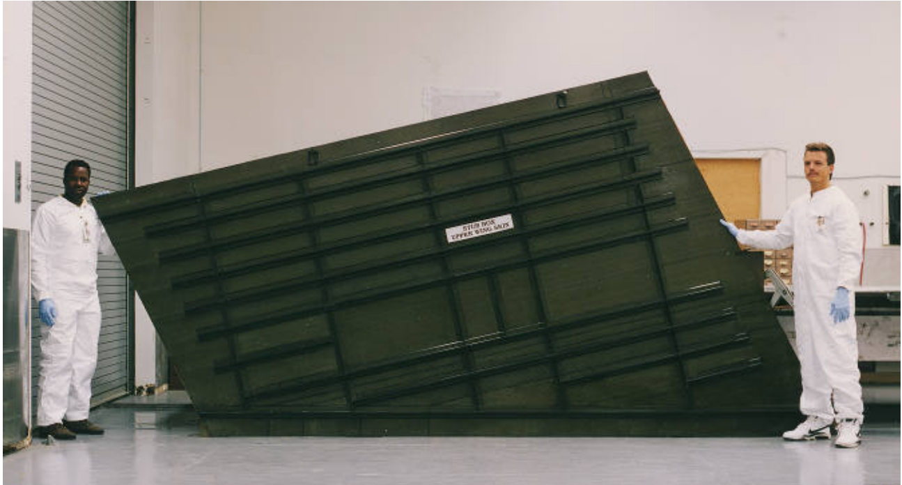
Figure 23. Stitched/RFI upper cover for wing stub box test component.
