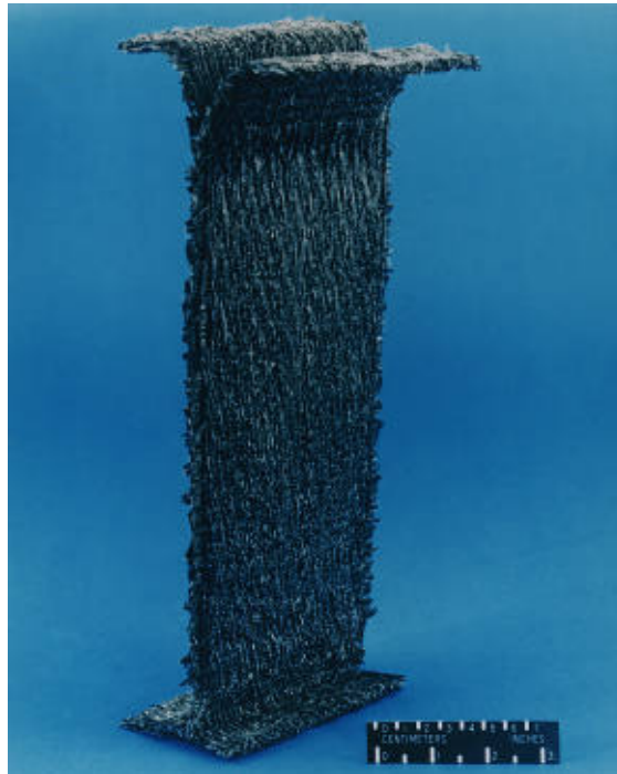
Figure 18. Woven preform (carbon-PEEK tow) for a wing Y-spar. (Northrop Grumman contract)
