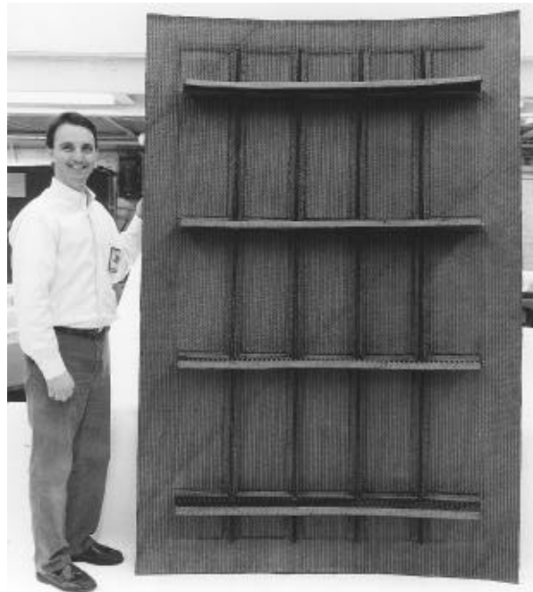
Figure 21. Cross-stiffened woven/stitched fuselage side panel.
