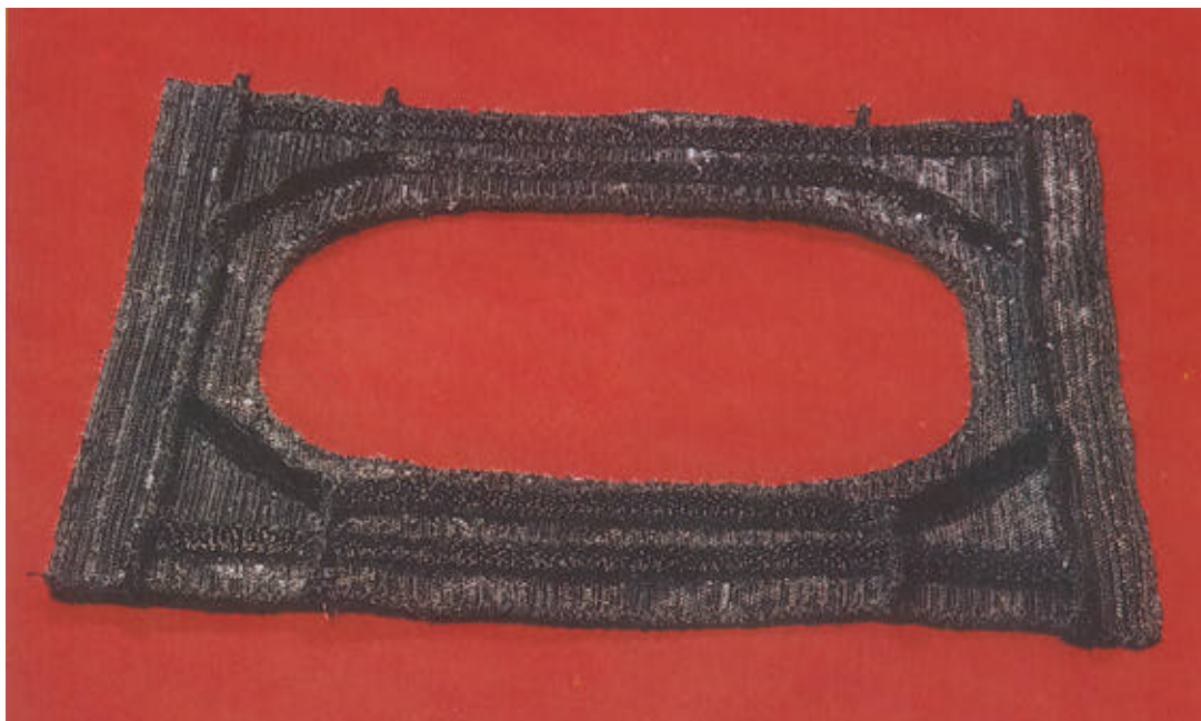
Figure 14. Three-dimensional integrally woven preform (epoxy-powder-coated tow) for a fuselage panel window belt component.
