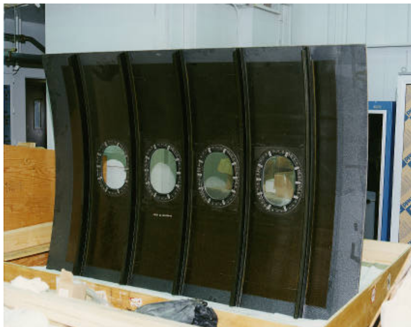
Figure 17b. Honeycomb-stiffened fuselage side panel with constant-section braided frames.
