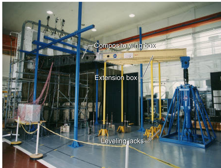
Figure 25. Stitched/RFI wing stub box test set-up at the Langley Structures and Materials Laboratory.
