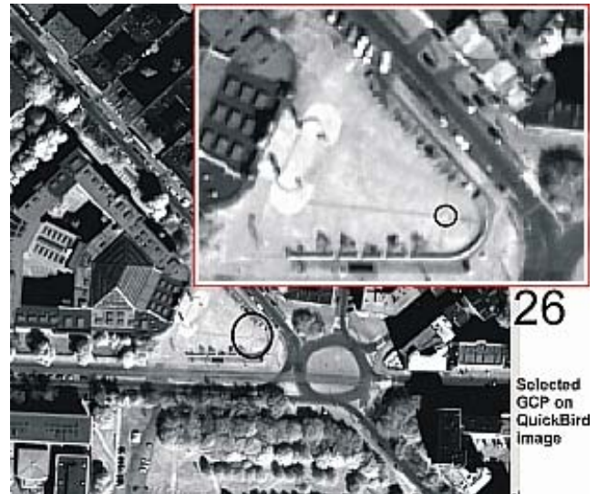
Figure 1. Projected identification GCP on QuickBird imaging fragment
