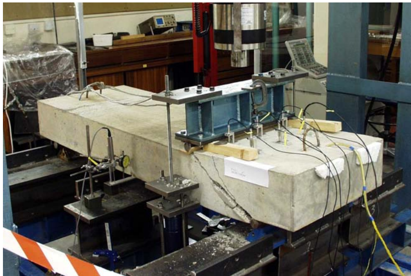
Figure 9: Bridge deck – shear test rig
