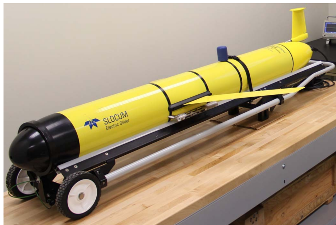
Fig. 1. A Slocum Glider with a double payload bay and a top-mounted acoustic modem in its deployment cart.
