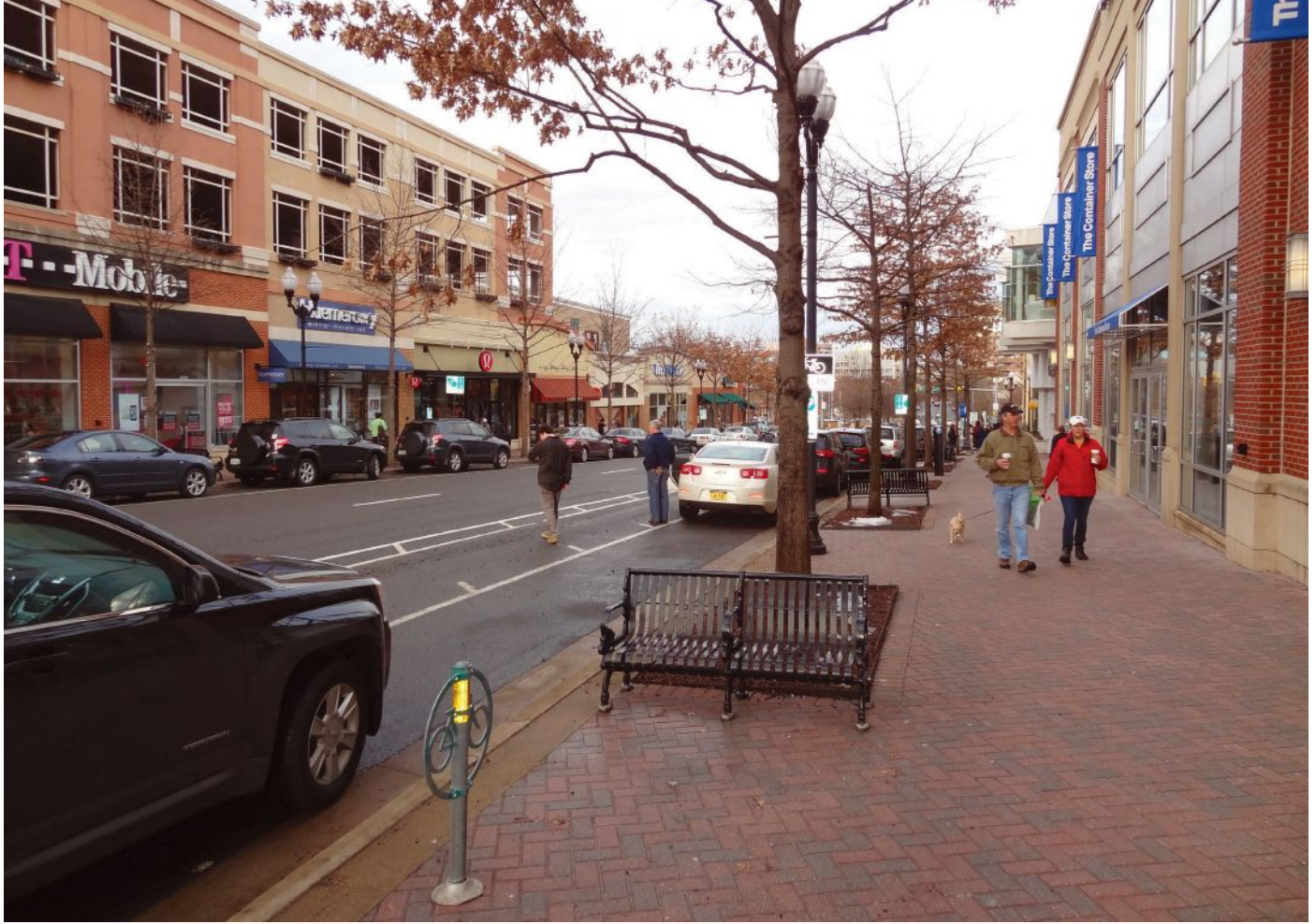
Clarendon Boulevard shows complete street features, such as ample sidewalks and pedestrian amenities; buffered bike lane; and two parking lanes and two travel lanes, reduced from three to make room for sidewalks and bike lanes.
