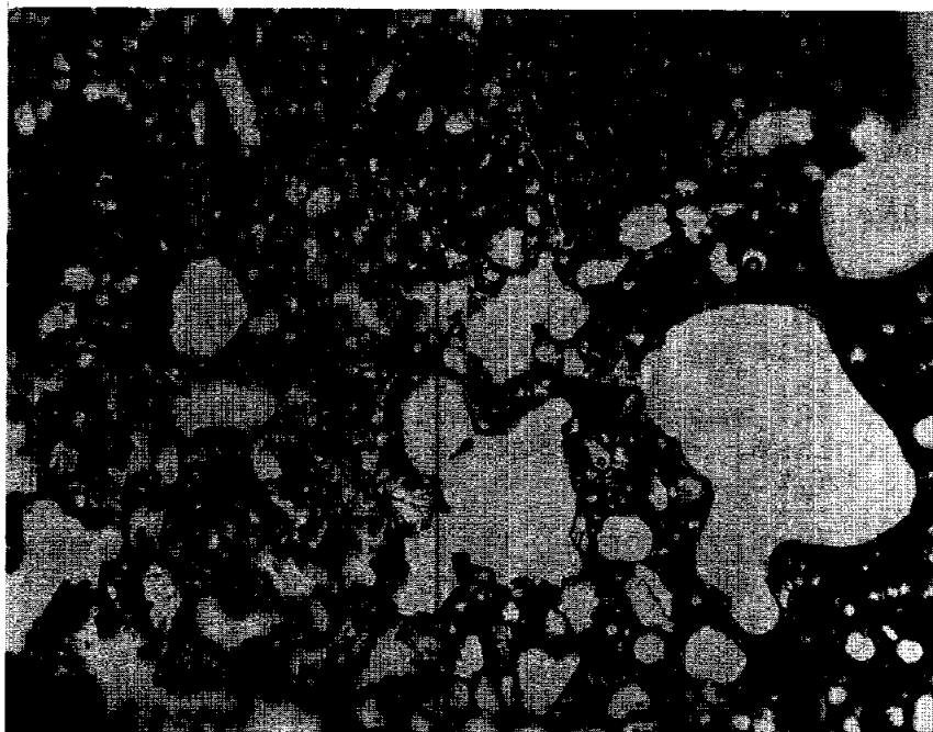
Figure 2. Photomicrograph of 15135,6, showing vesicles, fine matrix, and a melt clast. Width about 1.25 mm. Plane transmitted light.
