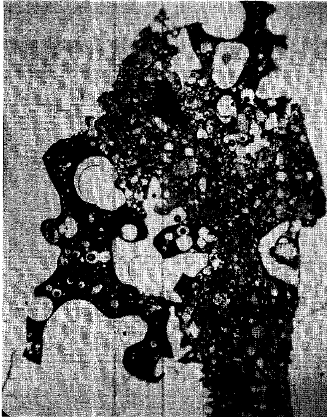
Figure 2. Photomicrograph of 15027,6. Width about 2 mm. Transmitted light. View shows both vesicular glass and glassy breccia.
