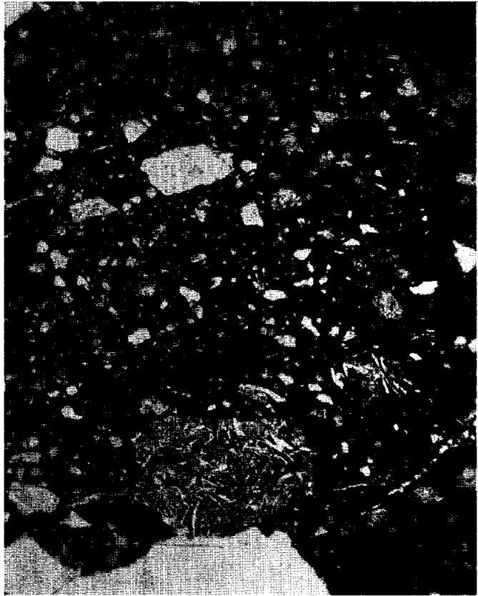
Figure 2. Photomicrograph of 15289,6. Width about 2 mm. Transmitted light. Clast in lower center is a mare basalt.
