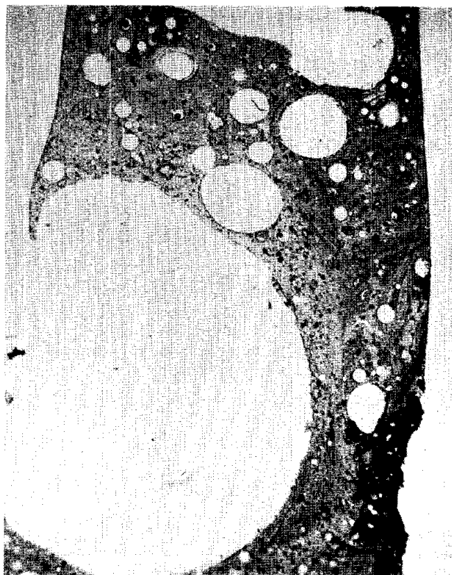
Figure 2. Photomicrograph of 15017,22. Width about 2 mm. Transmitted light. Section cut across shell; interior is to left.
