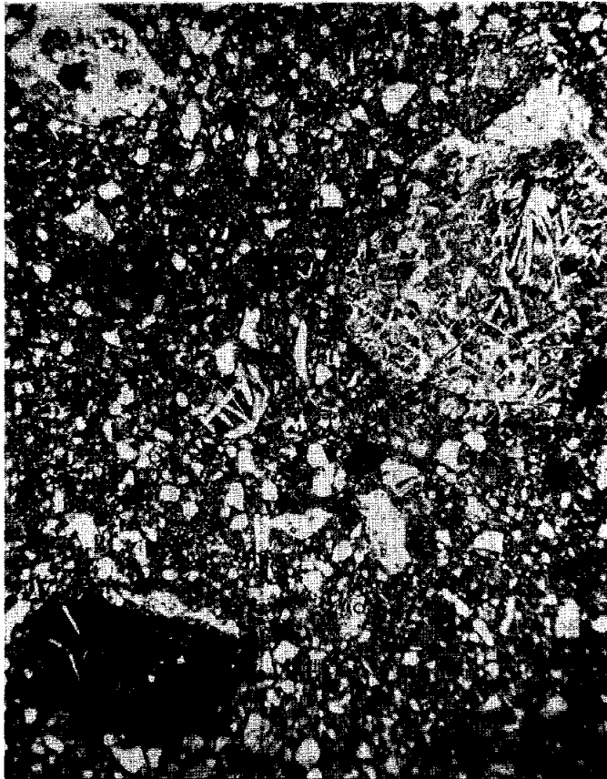
Figure 2. Photomicrograph of 15265,7. Width about 2 mm. Transmitted light. Basalt is an Apollo 15 KREEP basalt fragment.
