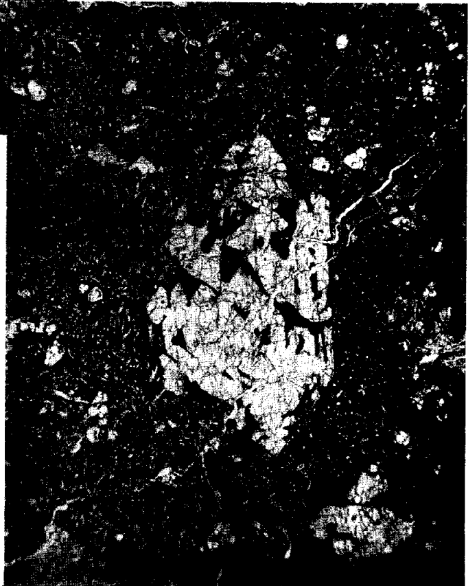
Figure 3. Photomicrographs of 15256,47. Transmitted light. widths about 2 mm. a) olivine-vitrophyric patch surrounded and intruded(?) by heterogeneous olivine-phyric, fine-grained basalt; b) zone of fine-grained basalt containing a large euhedral olivine containing patches of fine-grained to glassy melt; small phenocrysts are also olivine.
