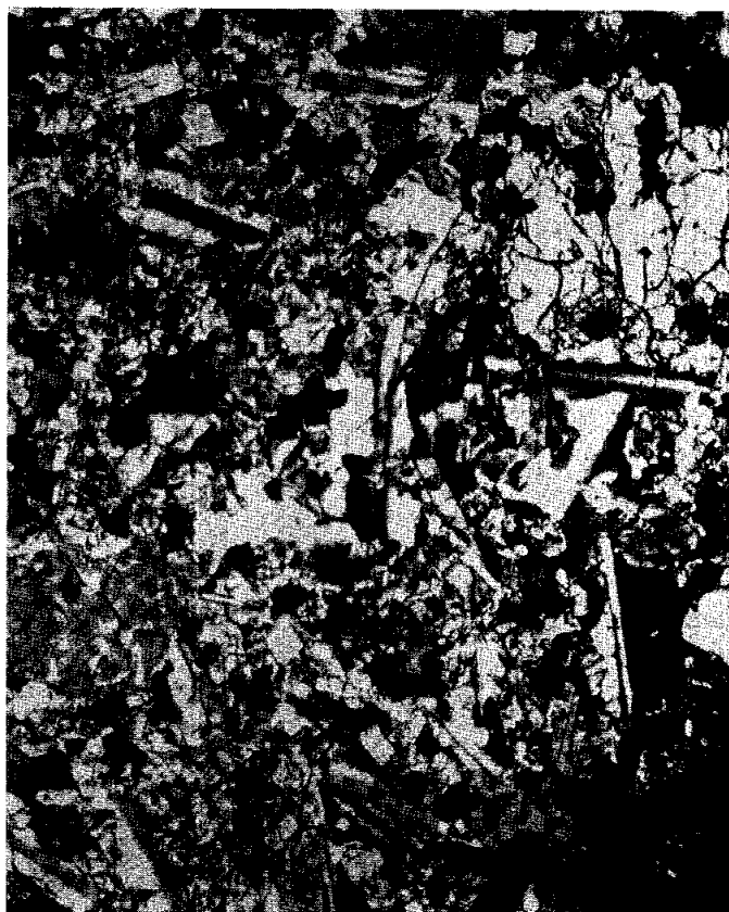
Figure 2. Photomicrograph of 15119,12 (a poor section) An olivine microphenocryst is on the center left edge. Crossed polarizers. Width about 1.25 mm.
