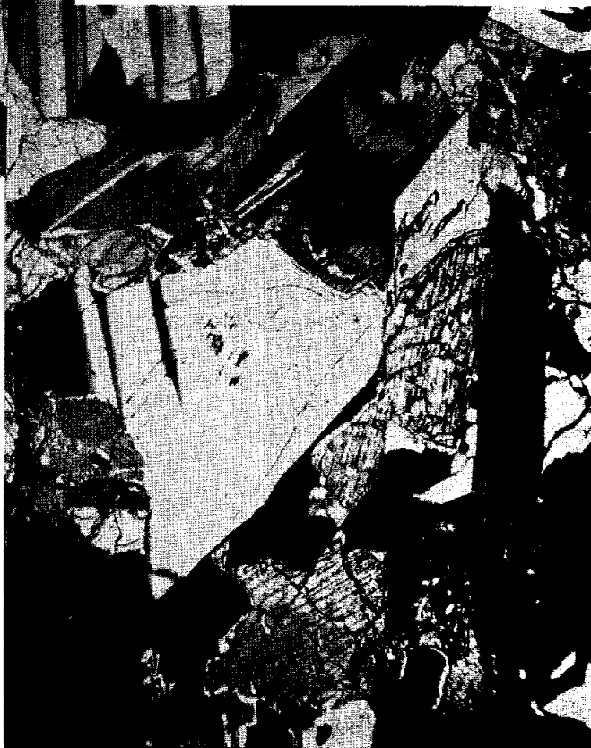
Figure 2. Photomicrographs of 15085,11. Widths about 3 mm. a)c) transmitted light. b)d) crossed polarizers. a)b) coarse groundmass with large plagioclases. Lath at right is tridymite. c)d) two zoned pigeonites (lower is twinned, and part of a 1 cm grain). Middle right are tridymite laths intergrown with opaque phases. Upper right are tridymite laths embedded in a 1 mm grain of pyroxferroite.
