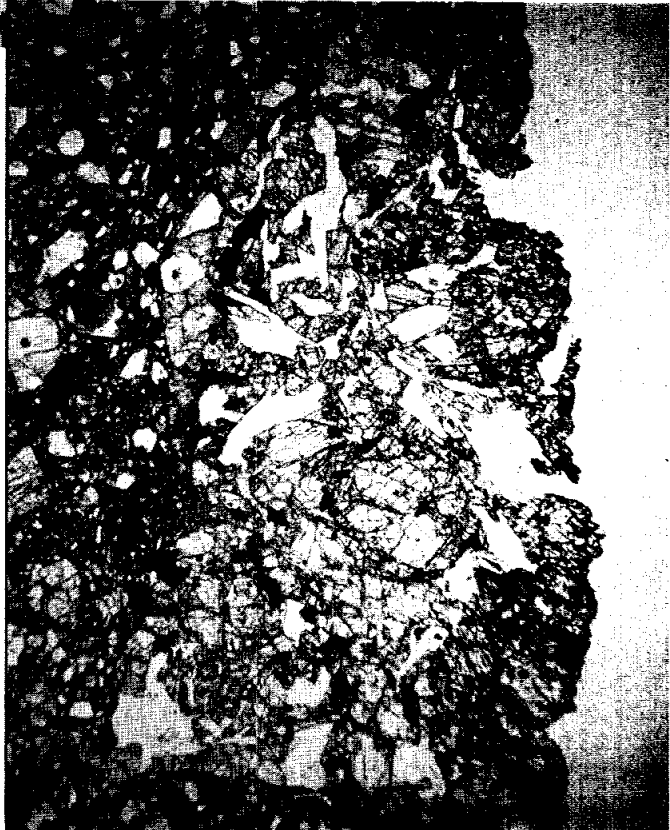
Figure 2. Photomicrographs of 15025,4. Widths about 2 mm. Transmitted light. a) general matrix; b) mare basalt clast; c) KREEP basalt clast.
