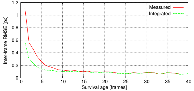
Figure 2. RMSE of inter-frame feature position as function of the survival age.
