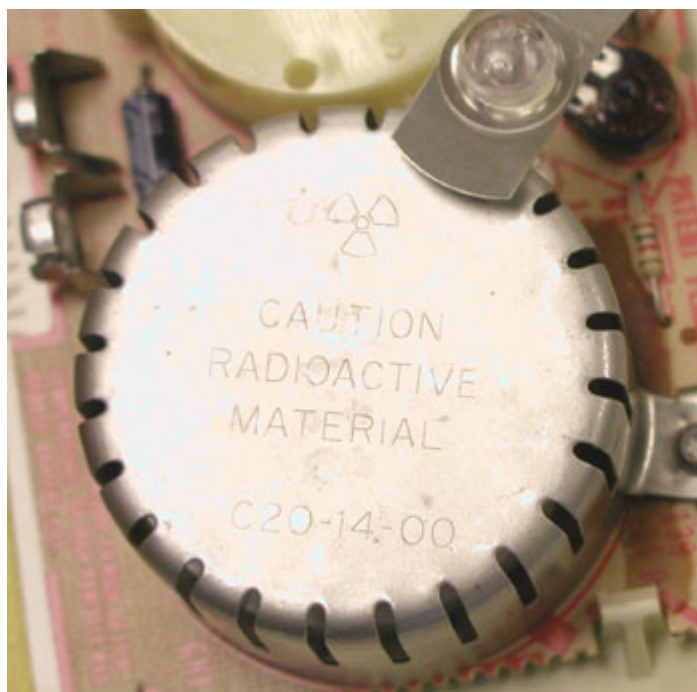
Figure 6.2 Am-241 Smoke Detector Source
