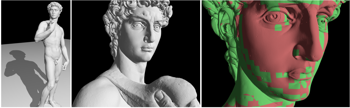
Figure 1: A 1 billion triangle model is rendered on a 1920 \times 1080 viewport using rasterization and ray-casting simultaneously. Ray-casting works on a sample-based surface LoD representation at an effective maximum sampling resolution of 8K^2 \times 32K . Red and green surface areas indicate parts of the model that are rendered via rasterization and ray-casting, respectively. On a GTX 680 graphics card the hybrid approach always renders the model in less than 30 ms ( > 33 fps) at a screen space error below pixel size.
