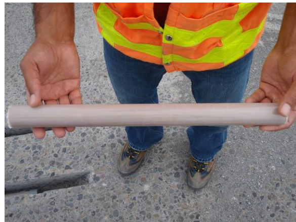
Figure 7. Close-up of GFRP dowel.
