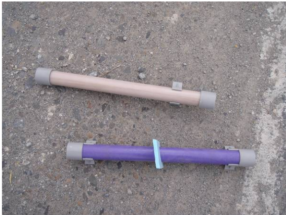
Figure 4. GFRP bar top, epoxy coated bar bottom.
