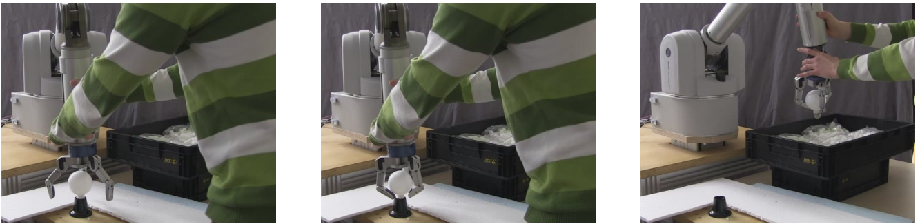
Figure 3.4.: Kinesthetic demonstration with a Barrett WAM. The skill of unscrewing a light bulb was taught to the robot by guiding its arm through the movement. Transitions between primitives were indicated by pressing a key. Also, the closing and opening of the hand was activated by pressing a key in order not to influence the force torque sensor at the wrist of the robot.
