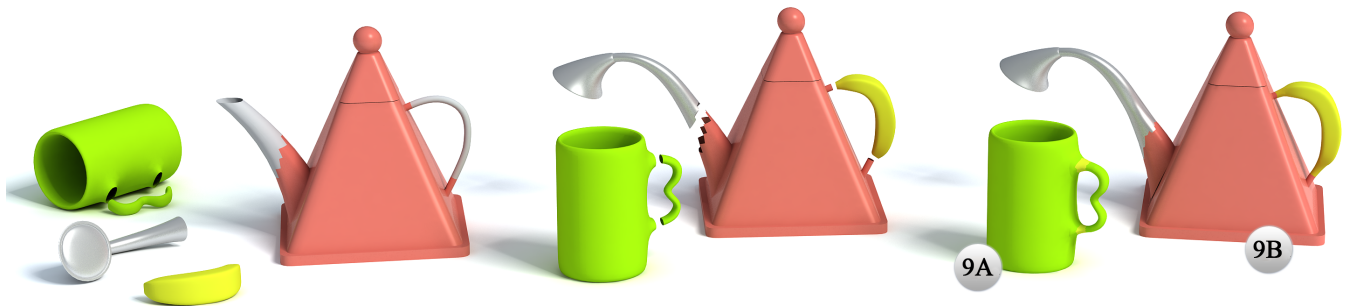
Figure 9: Composition of parts with more than one open boundaries. The parts come from the models on the left; in the middle we present automatic field-guided registration results, where the alignment step searches for a rigid transformation based on multiple pairs of open boundaries; the right side shows two final models obtained after gap filling.
