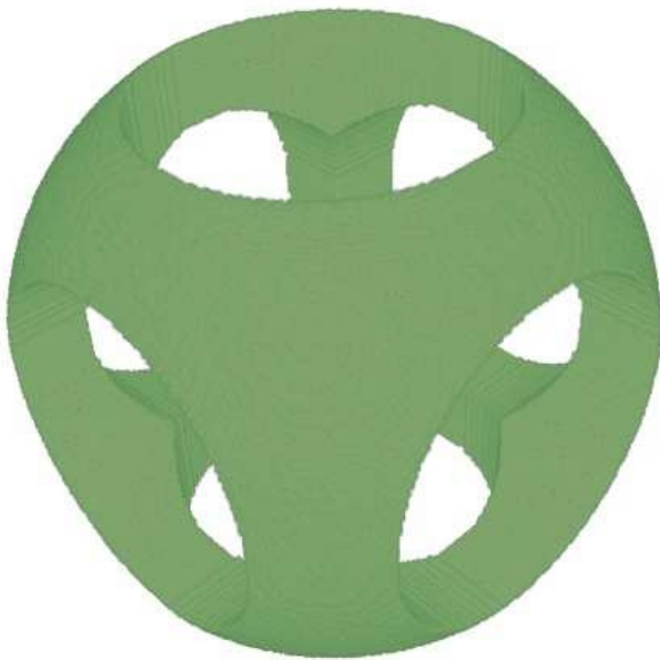
Fig. 5. Sphere and cylinders difference.
