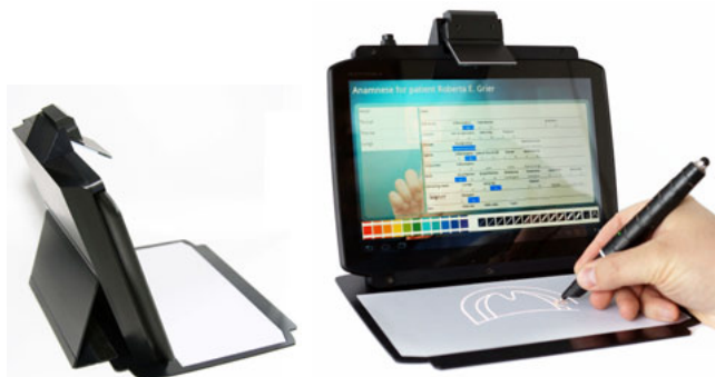
Figure 1. The Penbook setup: a mounted tablet computer with an integrated projector augments a paper screen that supports digital handwritten input transformed to projected light.
