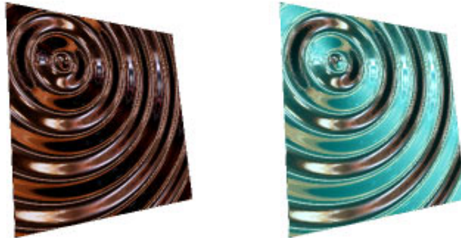
Figure 9.2: Combination of environment mapping and normal mapping. Left: environment map only. Right: local Phong illumination plus environment map.
