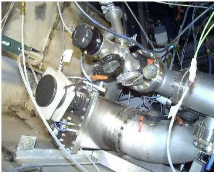
FIG. 42: The exit of the tagger vacuum box before modification. The beam exit pipe is the straight pipe exiting the figure in the middle of the right side. The background sources in this area such as small diameter beam pipe, flanges and pump out port are also shown.
