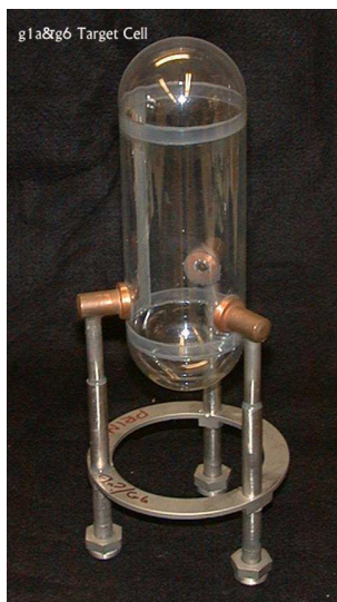
FIG. 29: TPE liquid hydrogen target cell. The mylar target cell is supported by hollow stainless steel legs with copper nozzles.
