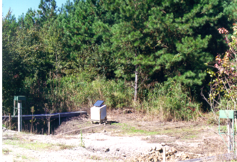
Figure 3. Typical flow station setup with stormwater sampler house, upstream stage recorder (left) and downstream stage recorder (right).
