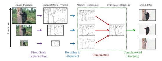
Figure 2. **Multiscale Combinatorial Grouping**. Starting from a multiresolution image pyramid, we perform hierarchical segmentation at each scale independently. We align these multiple hierarchies and combine them into a single multiscale segmentation hierarchy. Our grouping component then produces a ranked list of object candidates by efficiently exploring the combinatorial space of these regions.
