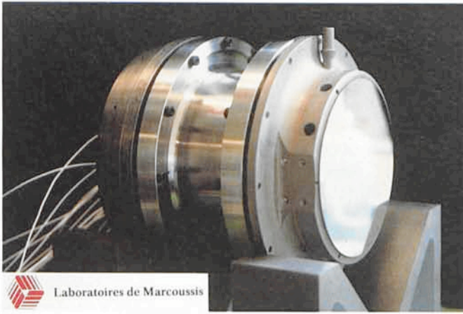
Figure 2: Deformable mirror developed at CGE-Laboratoires de Marcoussis with 19 piezoelectric actuators.
