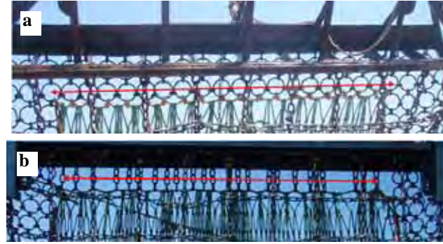
Figure 4: Example of methods used to hand the twine top: rings (a) and chains (b).
