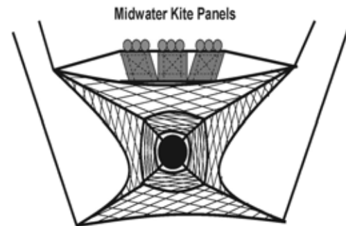
Figure 5: Orientation of kite panels. View looking into the mouth of the net.
