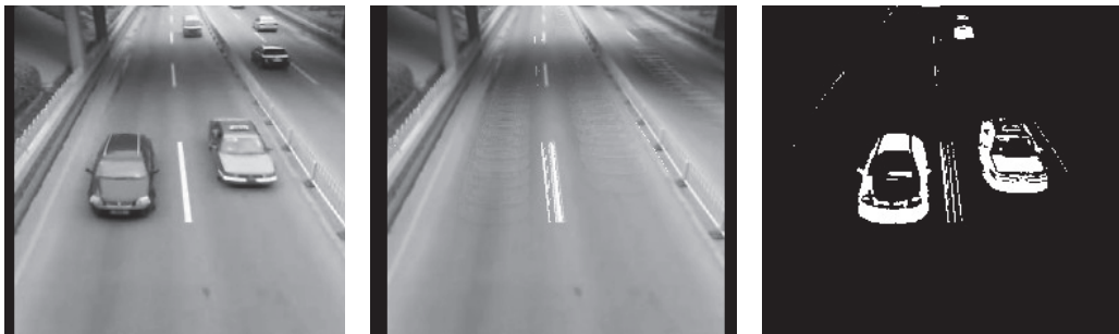
Fig. 7 Segmentation of moving vehicle: Left: present frame image Middle: background image Right: segmenting result of moving vehicle.
