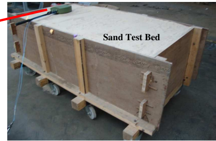
Figure 12. Sand test bed used for scattering experiment.
