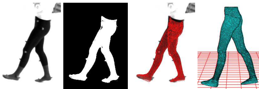
Fig. 9. From left to right: (a) Original image. (b) Silhouette. (c) Estimated pose. (d) 3D model.
