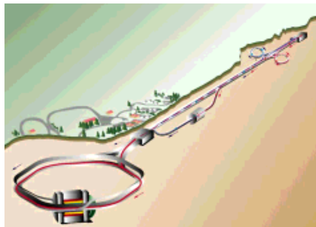
Figure 1: Overview of SLAC linear accelerator showing injection into the PEP-II asymmetric collider including the BABAR detector which is presently being installed.
