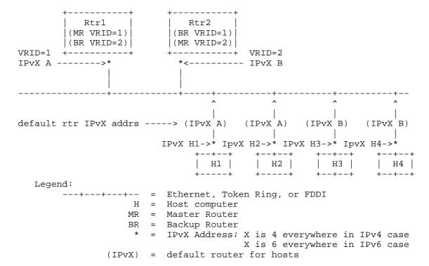
In the IPv4 example above (that is, IPvX is IPv4 everywhere in the figure), half of the hosts have configured a static route through Rtr1's IPv4 A, and half are using Rtr2's IPv4 B. The configuration of virtual router VRID=1 is exactly the same as in the first example (see Section 4.1), and a second virtual router has been added to
