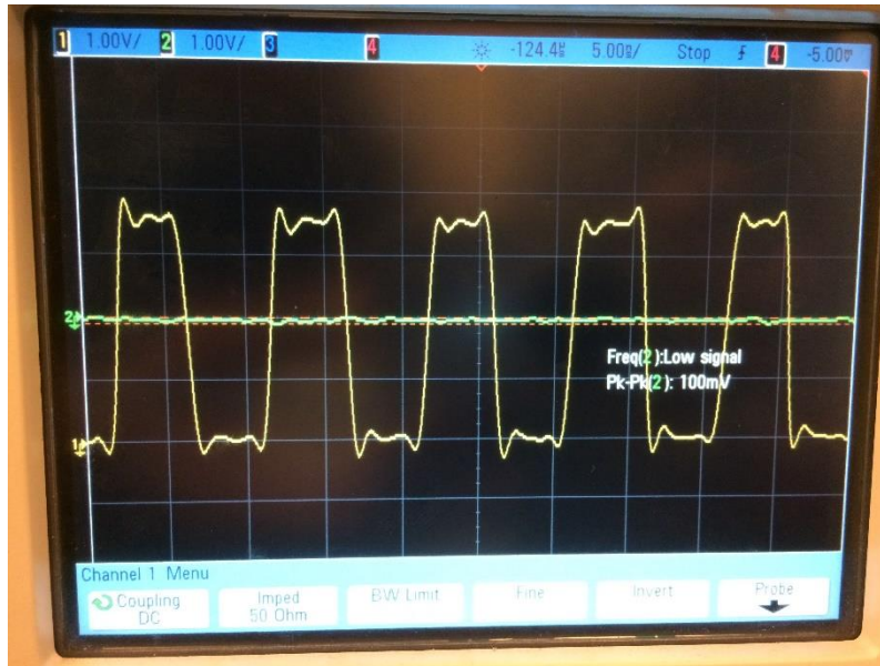
Fig. 5-67, Transient response of one of the cascode driver stages
