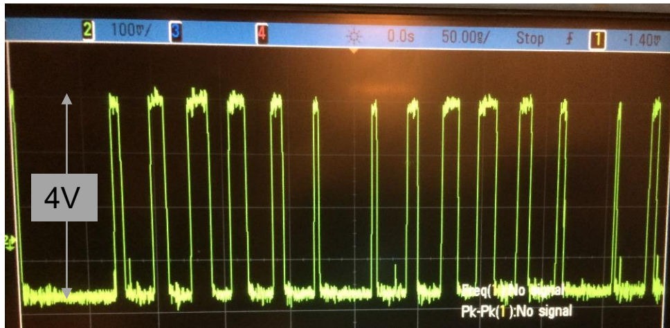
Fig. 5-64, Transient response of the HoC driver stage (after 20dB attenuation)
