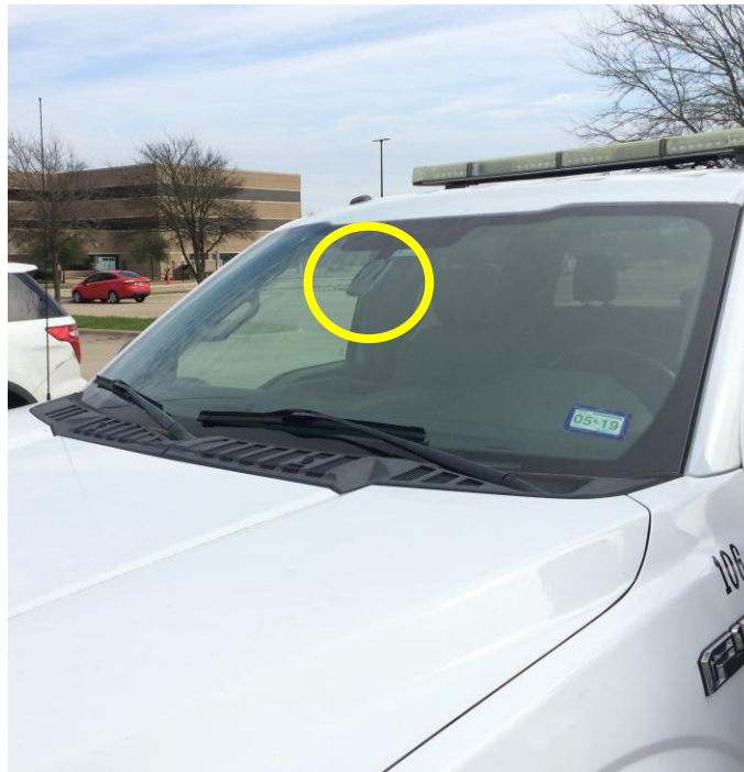
Figure 7. Machine Vision Camera Position on Data Collection Truck
