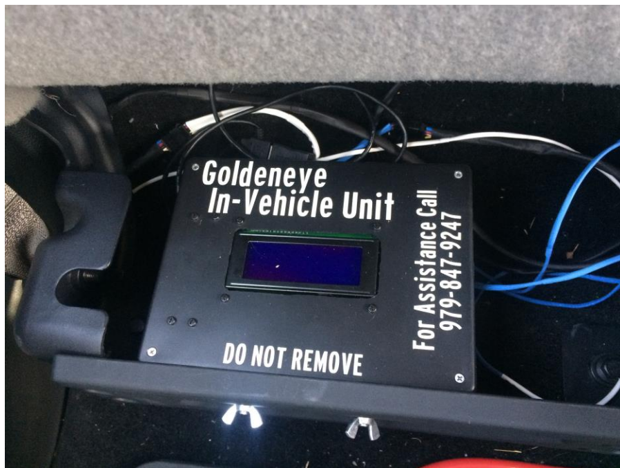
Figure 9. Machine Vision In-Vehicle Data Unit
