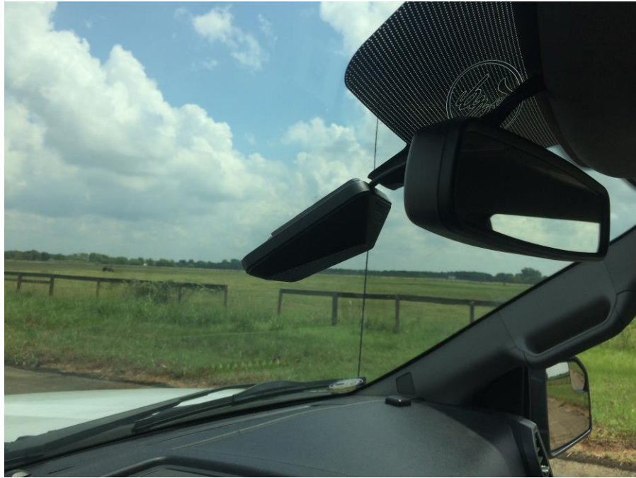
Figure 8. Installed Machine Vision Camera
