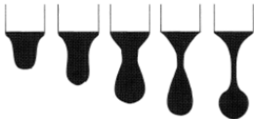
Figure S8. Schematic of the detachment sequence of a drop hanging from the tip of a capillary (Thermopedia, 2015).
