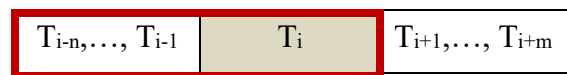
Figure 3.3 Prediction of a sequence of m data points by RNN/Bi-LSTM given data point at time-step T_i and its n past data points
