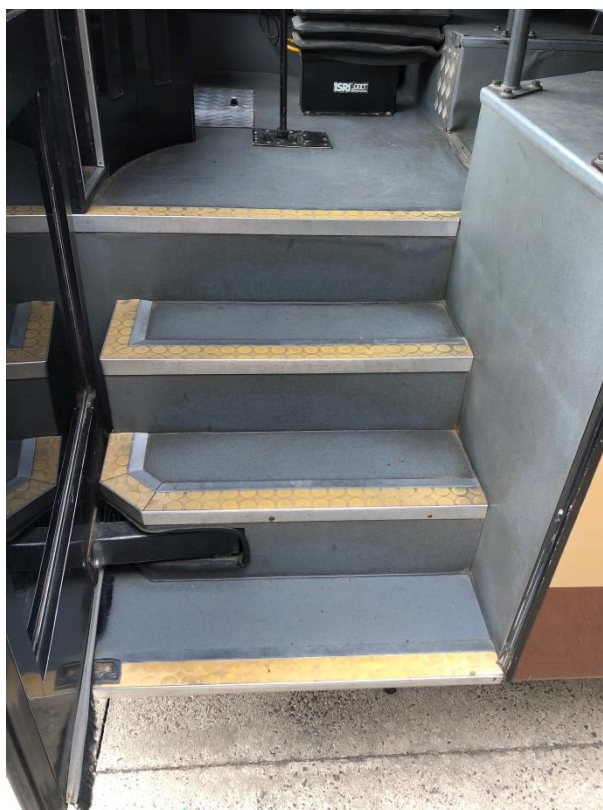
Figure 6-18 Bus entrance showing the steps and driver's seat landing
