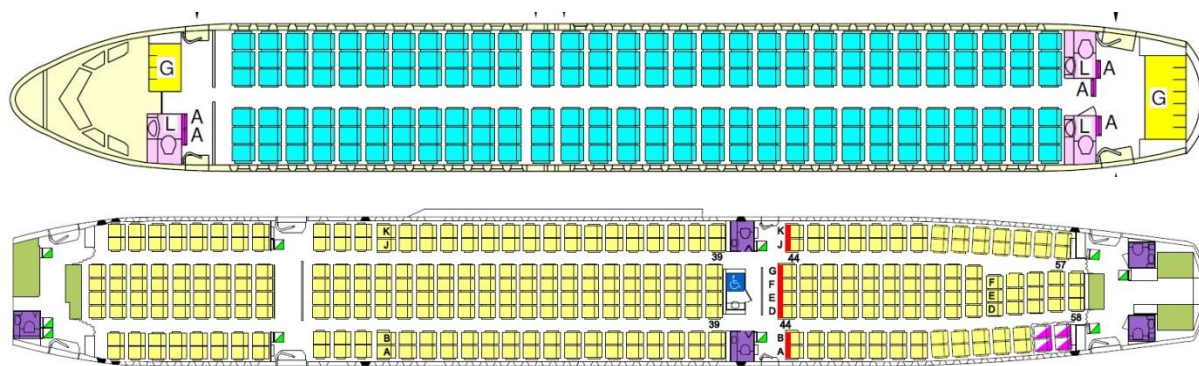
Figure 6-4 Cabin layout used for simulation for the A320 (above) and A330-200 (below) (Airbus, 2014; Airbus 2015)
