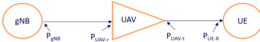
Figure 3.4: End-to-end representation of the gNB to the UE communication using a relay node.
