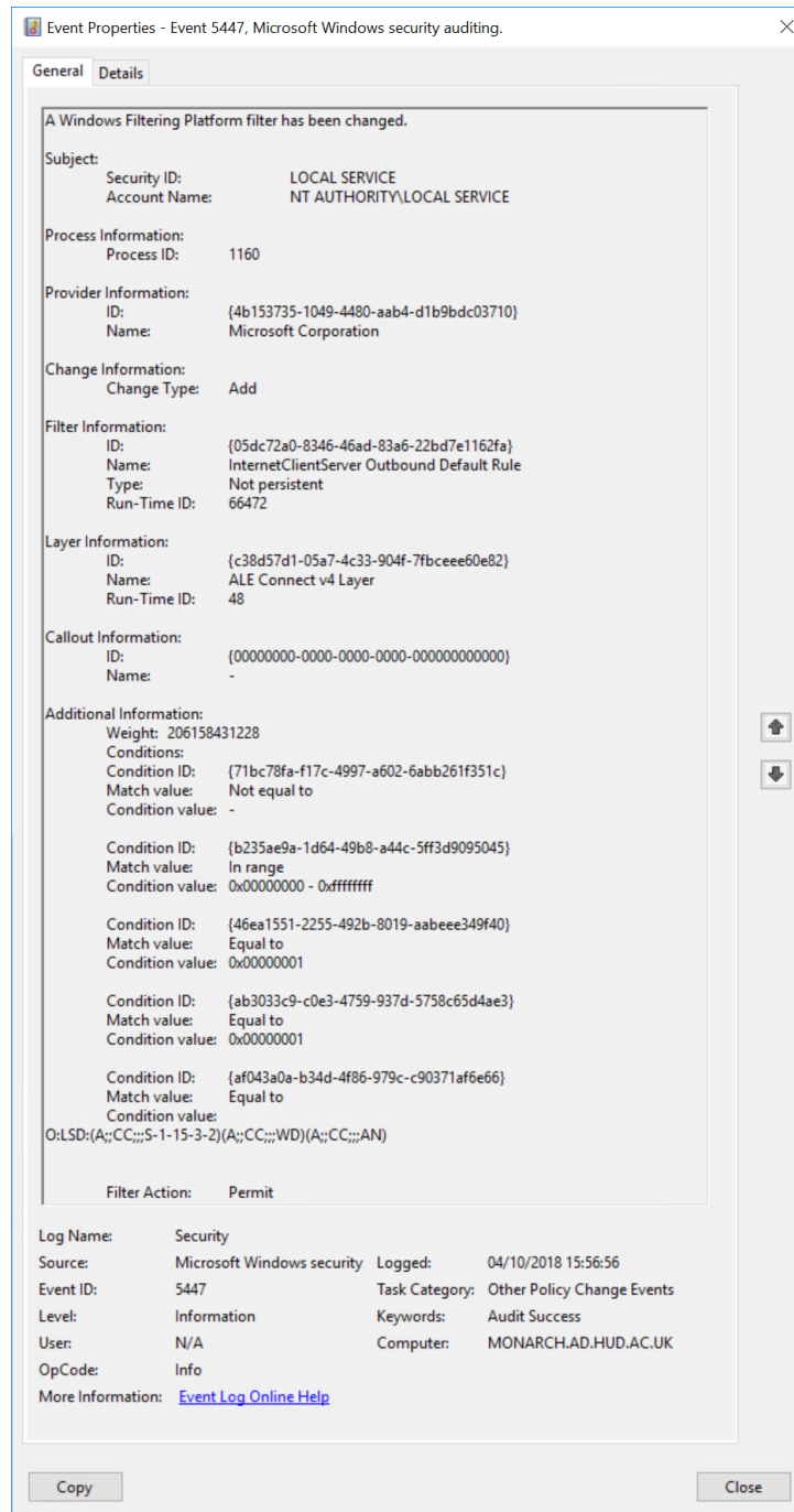
FIGURE 3.3: A live entry of event type, 5447, acquired using the Event Viewer application of a Microsoft system. It shows the description of event, list of all object-value pairs and other relevant information.
