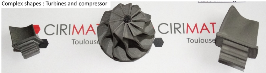
Fig. 16 Complex shapes part elaborated in one single SPS cycle.
