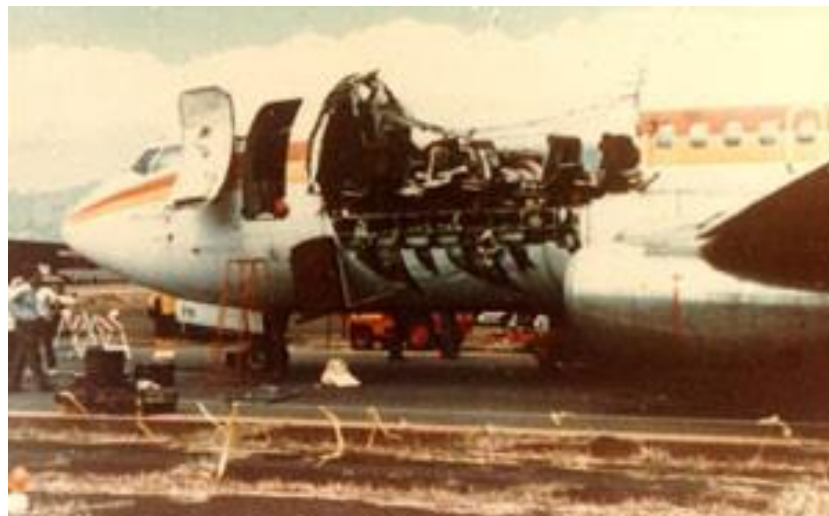
Figure 1-1: Photograph of the Aloha accident aircraft after landing. Front upper fuselage shell is damaged and was lost during flight due to Wide-Spread Fatigue Damage (WFD). (Photograph was taken from [4])
