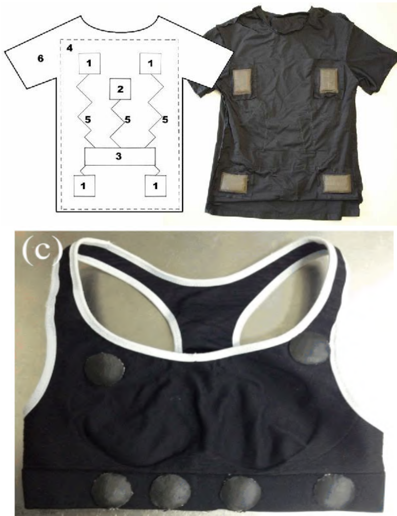
Figure 2.21 Examples of smart shirts for man and woman, respectively composed of textile and polymeric electrodes
