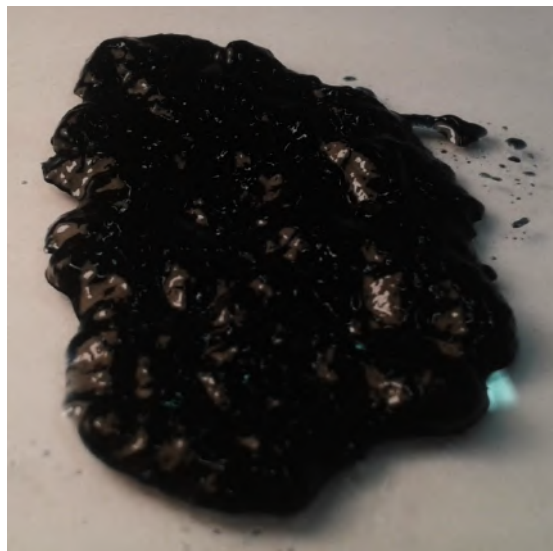
Figure 5.5 Conductive ink for screen-printing composed by PEDOT:PSS
