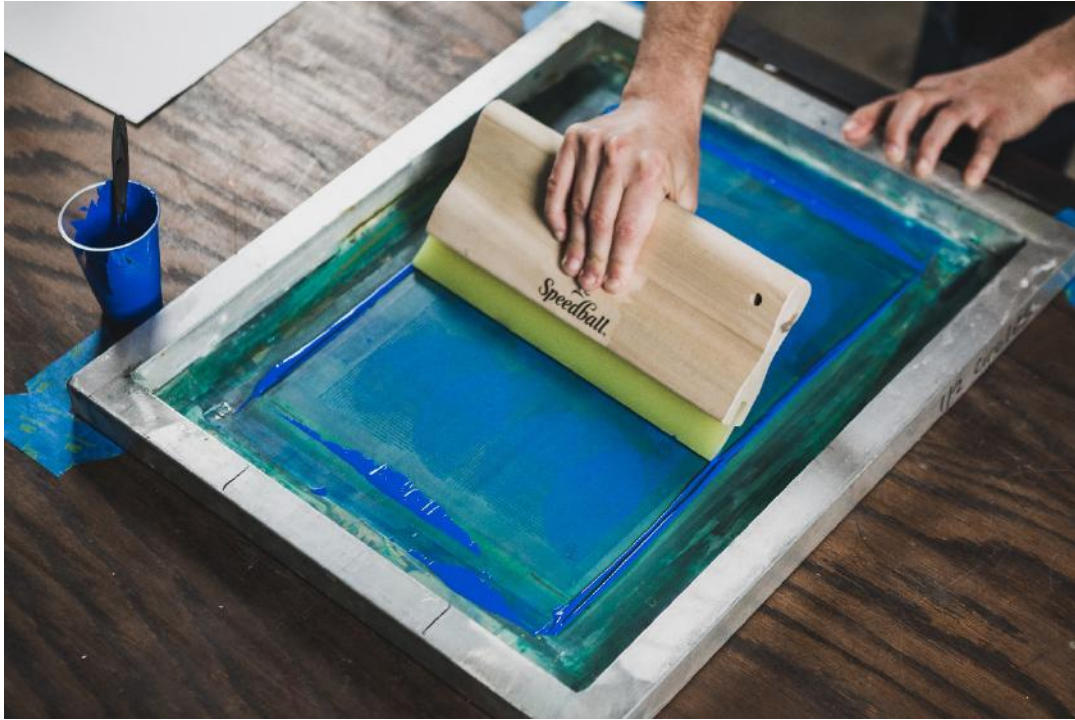
Figure 3.7 Screen-printing instrumentation composed of ink, frame and squeeze
