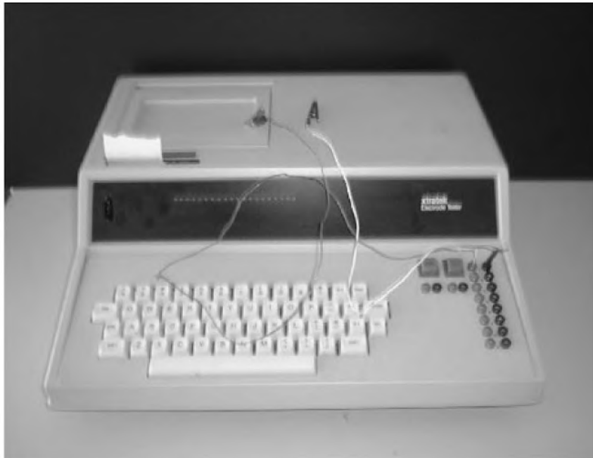
Figure 4.3 Xtratek ET-65A ECG electrode tester
